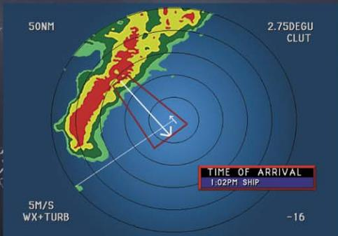
DOPRAD® 32 Display with Storm Path Analyzer
