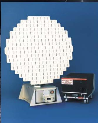
30" Flat Plate Phased Array, Pedestal, Mounting Bracket, and Receiver/Transmitter
